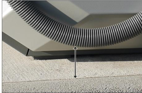
→ Adjust hose length on site. When the automatic nozzle is attached, the suction hose operator may not lay on the floor, and must therefore maintain a minimum distance of 5 cm to the floor. If necessary, adjust the length of the double casing suction hose.
